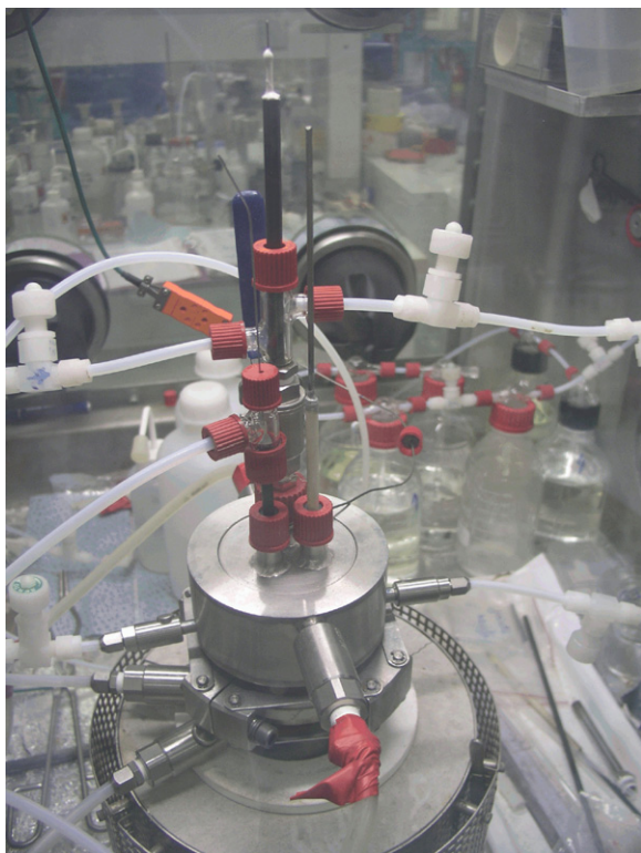
Fig. 3. Electrochemical cell in the glovebox (Atalante facility, Marcoule, France).
